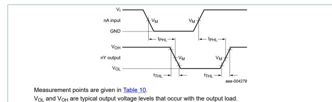
Fig. 6. Propagation delay data input (nA) to output (nY) and output transition time
