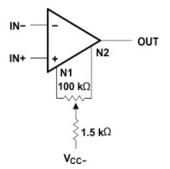
Figure 7-3. Input Offset-Voltage Null Circuit
