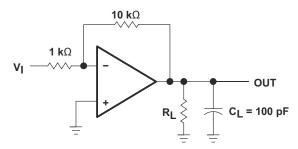
Figure 7-2. Gain-of-10 Inverting Amplifier
