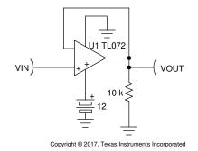
Figure 9-3. Single-Supply Unity Gain Amplifier
