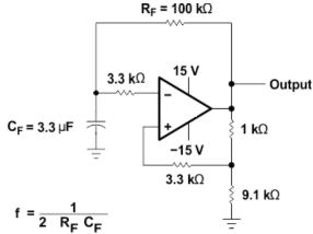
Figure 9-6. 0.5-Hz Square-Wave Oscillator
