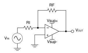
Figure 9-1. Inverting Amplifier
