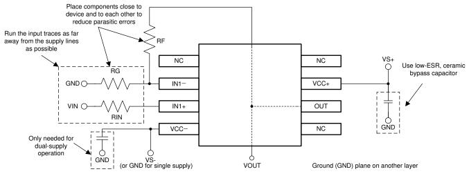
Figure 11-1. Operational Amplifier Board Layout for Noninverting Configuration
