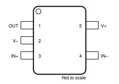
Figure 5-1. TL071H DBV and DCK Package 5-Pin SOT-23, and SC70 Top View
