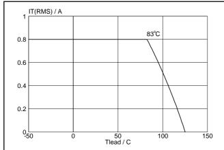
Fig.3. Maximum permissible rms current  $I_{\text{T(RMS)}}$  , versus lead temperature,  $T_{\text{lead}}$ .
