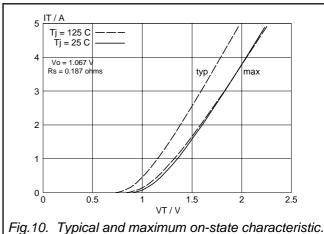
Fig. 10. Typical and maximum on-state characteristic.
