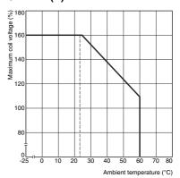
Note. The maximum coil voltage is the maximum voltage that can be applied to the relay coil.
