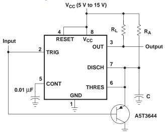
Pin numbers shown are shown for the D, JG, P, PS, and PW packages.
