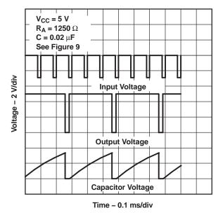
Figure 17. Divide-by-Three Circuit Waveforms
