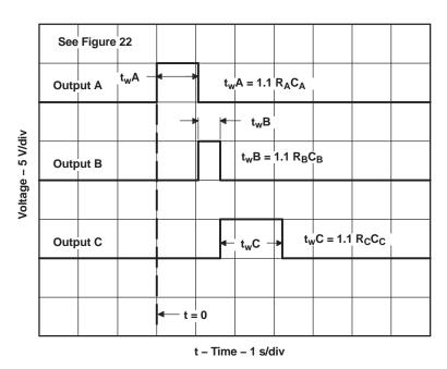
Figure 23. Sequential Timer Waveforms
