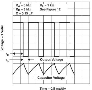
Figure 13. Typical Astable Waveforms
