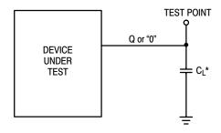
\*Includes all probe and jig capacitance.
