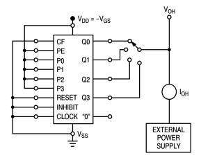
Figure 1. Typical Output Source Characteristics Test Circuit
