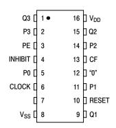
Figure 1. Pin Assignment
