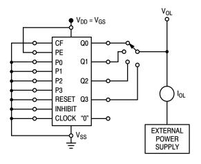
Figure 2. Typical Output Sink Characteristics Test Circuit
